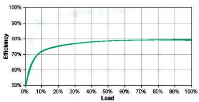
Curve fit to measured runtime data. All measurements taken with new, fully charged batteries, at typical environmental conditions, with no electrical input and balanced resistive load (PF = 1.0) output.
